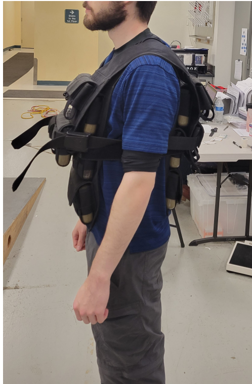
Figure 4: Carried Load consisted of bars of lead strapped in V-max weight vests. Pictured: 85lbs carried load, bottom vest carrying 50lbs and top vest carrying 35lbs.
