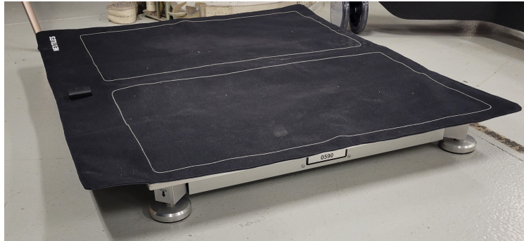
Figure 8: An example of the Nextiles sensor stacked on top of the Hawk Dynamics force plate for testing.
