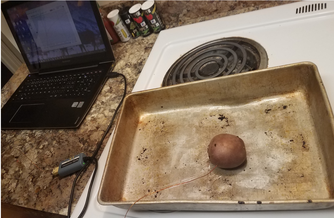
Figure 3: Data Acquisition Setup for Baked Potato on a baking sheet. Contact with the baking sheet will have altered heat transfer.
