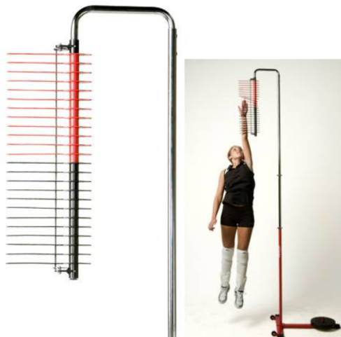
Figure 2: This is a mechanical measurement device for the vertical jump height [5], one common device replaced by the force sensors in figure 1 and the metric examined in this experimentation.
